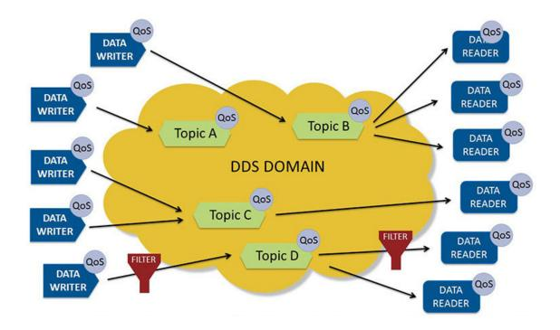
DDS provides QoS-controlled data-sharing. Applications communicate by publishing and subscribing to Topics. Subscribers can specify time and content filters and, thus, get only a subset of the data being published on a Topic and only when it is needed.
