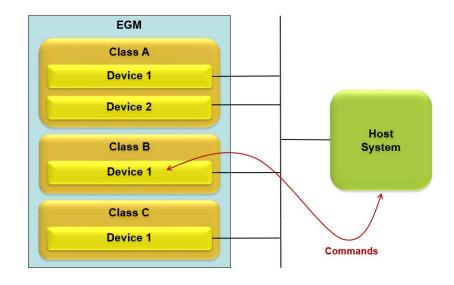
Two special classes are used to report meters and events for all classes. The meters class is used to report meter information. The eventHandler class is used to report events.
