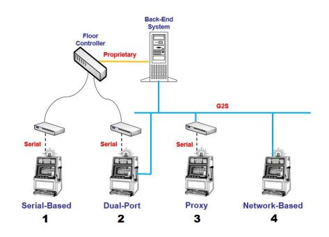
The left side (#1) displays where non-G2S systems are today: EGMs communicating over a serial communications line to an interface board, up to the floor controller, and eventually to the back-end systems.
