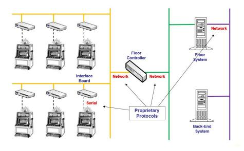
Advanced features, such as software download and remote configuration are impractical (or impossible) using such protocols. As demand for such features increased, it became evident that a network-based protocol with significantly higher bandwidth was needed to eliminate the bottlenecks and simplify the topology. Enter G2S.
