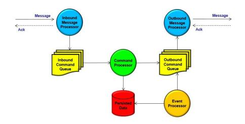
The *command processor* is where the application-level processing takes place. The command processor can prioritize and dispatch commands if necessary. The responses are placed in an outbound command queue.
