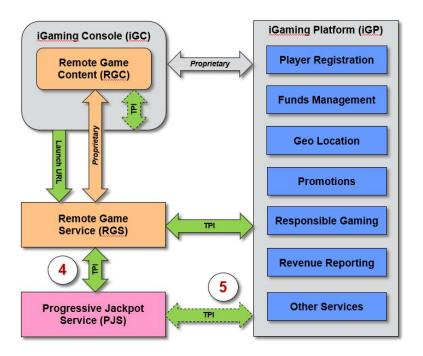
All commands in TPI are constructed using JavaScript Object Notation (JSON). Two message transport options can be used; JSON over Web-Sockets, or JSON over HTTP. For more information see "Command Structure & Game Launch URL" on page 19.
