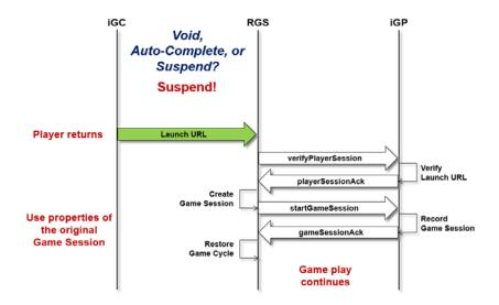
First, the iGC should send the game launch URL to the RGS as usual. The RGS should then verify the game launch URL as usual — the set of launch parameters contained in the launch URL should be sent to the iGP for verification.
