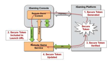
Prior to launching a game, the iGP generates a secure token (#1), recording the secure token and the associated launch parameters in its database.
