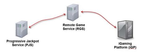
Configurations can be much more complex. Any of the three end-points can be comprised of multiple physical servers. Or a single physical server can host more than one service – for example, an RGS and a PJS can reside on the same physical machine.
